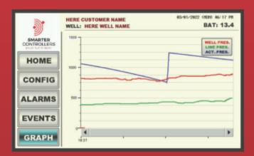
Graphics screen, allow you to know the pressures of the well and actuator in real time and also the historical data stored in the ESD-211 Controller.
