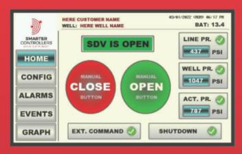
Main screen, allow you to operate, view the status of the SDV and the measured pressures.
